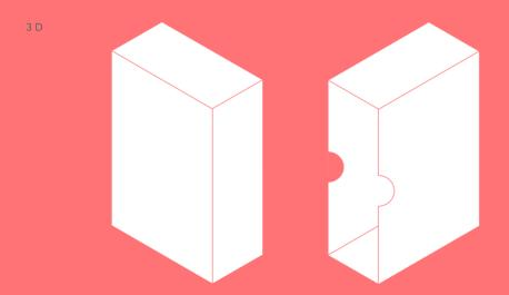
The size of the slip case is always based on the size of the book, which is to be kept inside. Construct the case out of a 270gsm – 300gsm paper/card.
